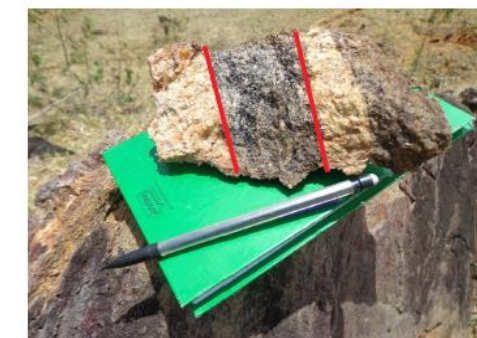
Photo 1 - Kinzigite Gneiss, featuring mineralized band in REE (La, Ce and Yb). Coordinates: X 431311 / Y 8141610 (SD24).
